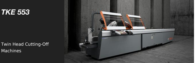
Twin-head cutting-off machine with 3 controlled axes, automatic traverse of the moving cutting head and electronic control of every angular setting from 45° (internal) to 15° (external) with accuracy of 280 places on each degree. The blade feed is controled by two hydro-pneumatic cylinders.
