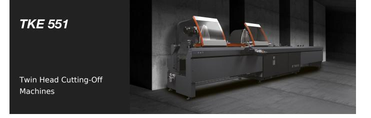
Electronic twin-head cutting-off machine with automatic traverse of the moving cutting head powered by brushless motor with numerical control system. Pneumatic control of the angular setting from 90° to 22°30' (external) with mechanic adjustment of intermediate angles. Hydro-pneumatic blade feed.
