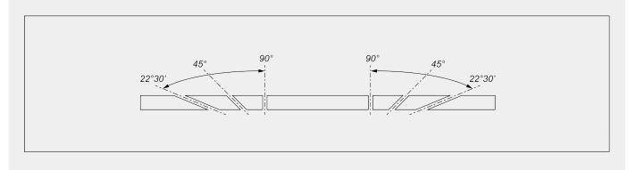
Mechanical adjustment of intermediate angles
