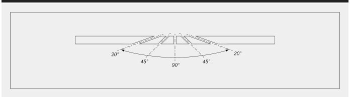
Mechanical adjustment of intermediate angles
