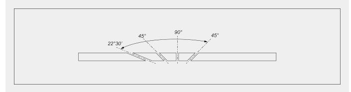
Mechanical adjustment of intermediate angles
