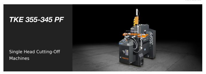
Single head cutting-off machine with horizontal blade feed and left loading side, pneumatic double side tilting of the cutting head in fixed positions: 45° to the left plus 90°, 45° and 22°30′ to the right. A special positive stop also allows cutting atintermediate angles.
