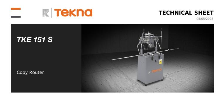
Single-head copy router with manual downfeed. Manually controlled single-head copy router with pneumatic clamping and traverse of the cutting head with indirect lever. Predisposition for performing through machining operations on aluminium without turning the workpiece and for working steel up to 2 mm. Scratch-proof work table. Pneumatic stylus with control on the handle.
