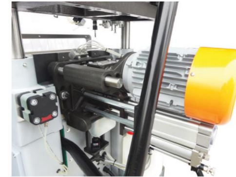
Back drilling unit
