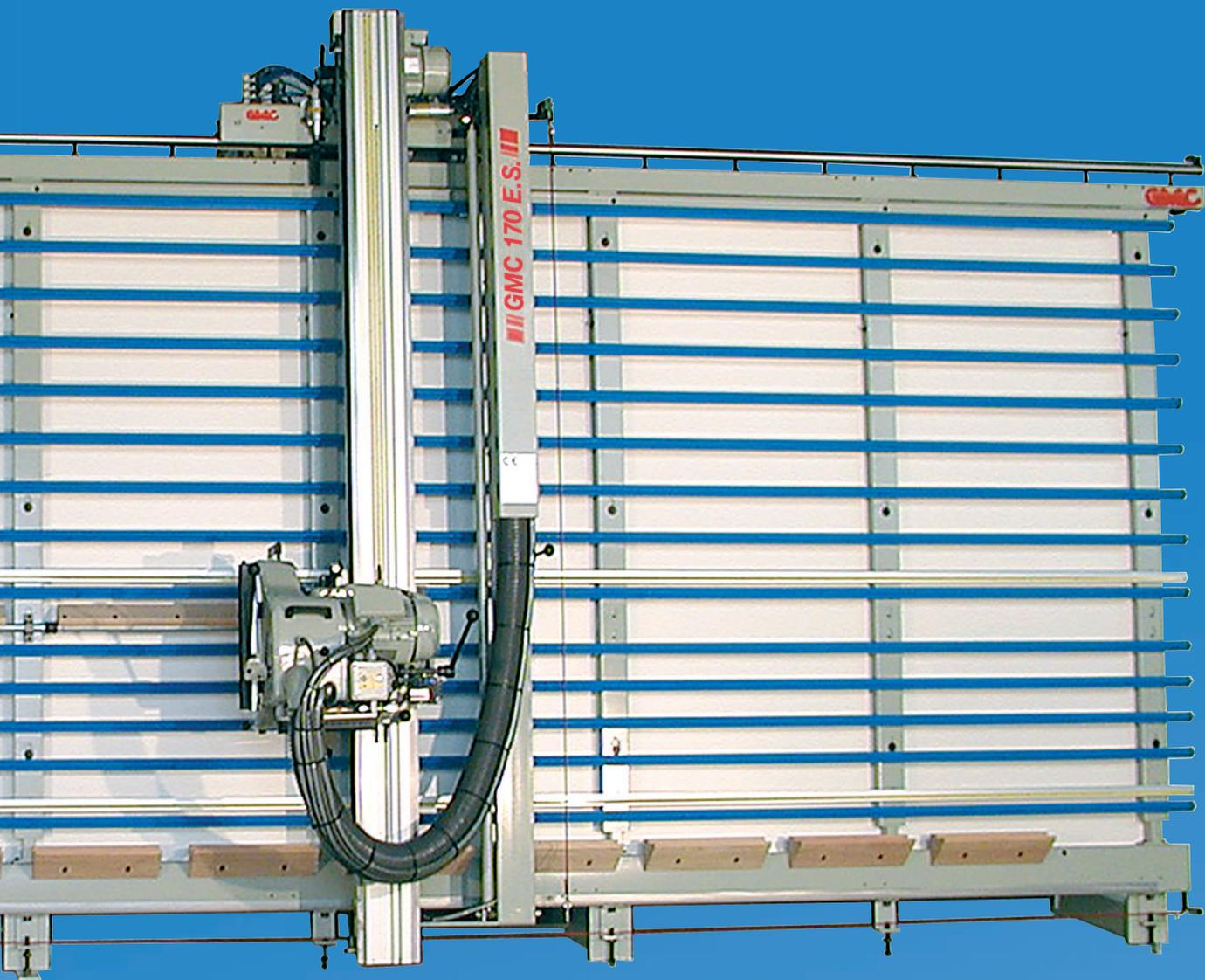
**VERTICAL PANEL SAW WITH ELECTRONIC PROGRAMMER FOR VERTICAL AND HORIZONTAL CUTS AND AUTOMATIC 90° SAWING-UNIT ROTATION.**
