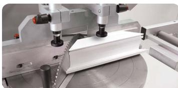
For cutting of aluminium and PVC profiles with a large cutting range
