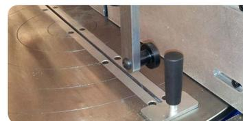
Manual intermediate angle adjustment according to scale, clamp-on design
