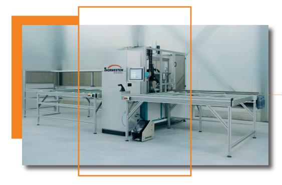
In the modular machining centre, all important components such as controller, monitor-based user interface, scanner as well as infeed and exit transport buffer are logically arranged. The superstructure of the PBZ profile machining centre is accessible from all sides, thus guaranteeing fast tool changes, as well as easy maintenance and repair.
