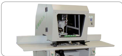
Option - sound insulating hood including gas pressure absorber for comfortable opening
