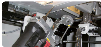
Drilling/milling unit from below with angle adjustment 0 - 65°
