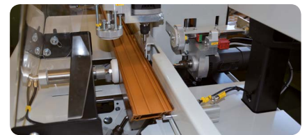
Pneumatic profile stops (left and right)
