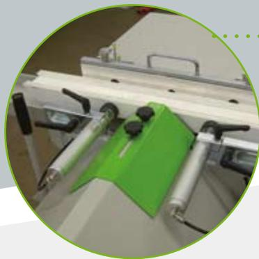
Fast fixing of the profile bar with a horizontal clamping cylinder (operated via foot switch).
