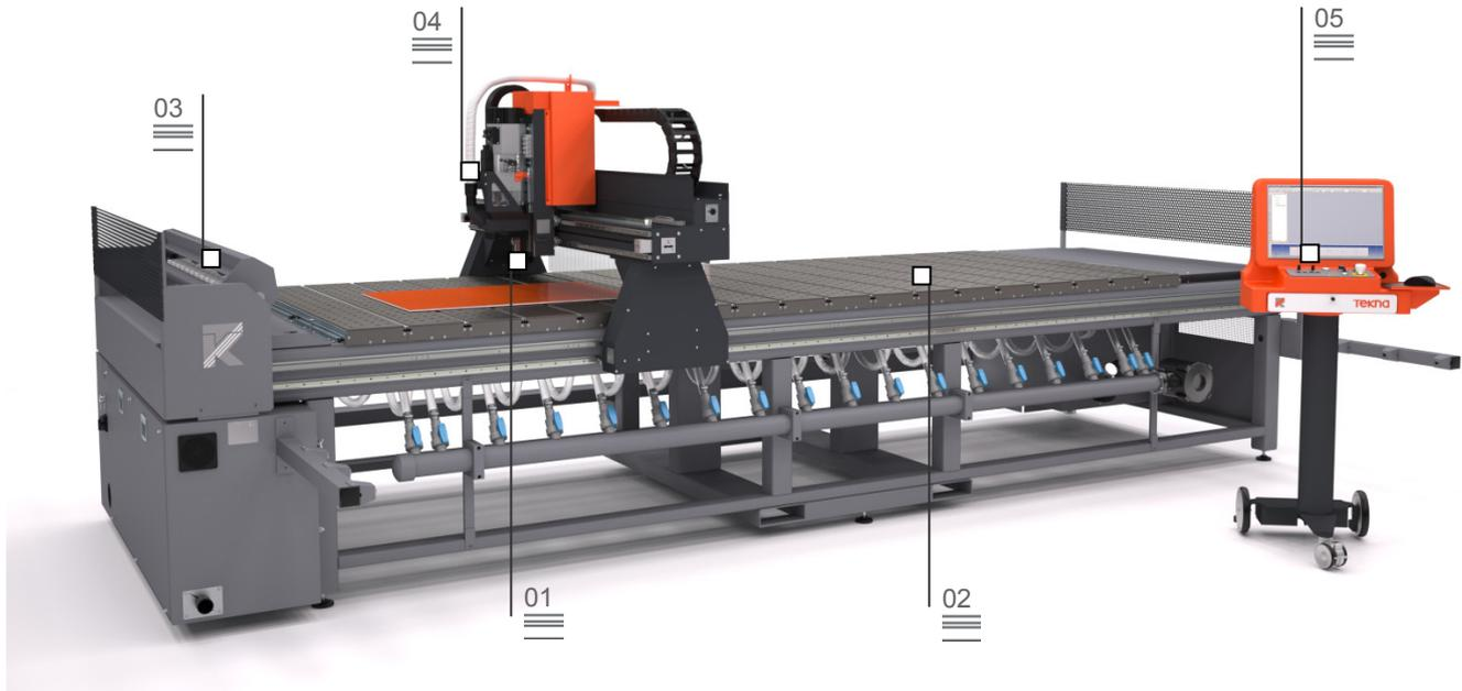
Vertical CNC machining centre with 3 controlled axes, including clamping system consisting of breather tables that anchor the panels and sheets by vacuum; this solution is particularly effective when machining thin components which are difficult to lock into position with conventional clamp systems.
